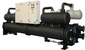
Falling film ground source heat pump Environmental refrigerant: R134A Rated cooling capacity range : 247-1971kW
