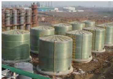
Large FRP storage tank Specification: DN100~DN4200、0.5~125m3
