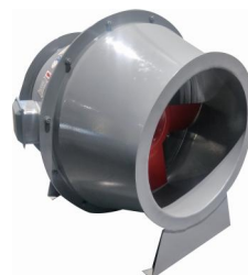
SJG Oblique flow duct ventilator Model: 2-8# Air volume: 260-25120m 3 /h Air pressure: 55-960pa
